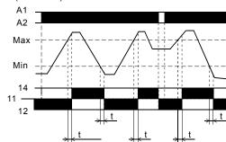
Note: the time delay t can prevent relay from maloperation in case of liquid level fluctuation.
